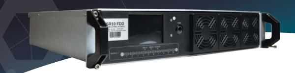
The SR-10-FDD is a Fiber High Density Desktop Dock offering. This unique desktop solution is designed to deliver 10 desktop computers over a tempest rated fiber in a 2U standard 19" rack configuration. Networking and power has been designed to deliver classified networks in one 2U shelf. Each desktop is designed to deliver KVM access through single fiber LC connection over a maximum distance of 20 KM. The SR-10-FDD has slots capable of receiving up to 10 BioDigitalPC® computers.
