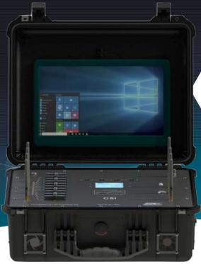
The MDC-C5i is a 30lb. portable data center and cyber, command, control, communications and computing solution holding 10 server cards with 10TB of total storage. The MDC-C5i has multiple options for connectivity including WiFi, 4/5G LTE, and Satellite/VSAT (optional). Each unit has 2×10 GE SFP+, 1×1 GE SWMGT, 1×1 GE AUX, 1×1 GE PWR MGT, 8×1 GB POE.
